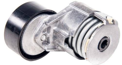
Control is then returned to the linear axis which applies enough force to hold the assembly together while a riveting head seals the finished tensioner. The final step is a controlled “unwinding” of the spring by the rotary axis to return the assembly to the “home” position without allowing the spring to snap back violently and potentially damage the completed tensioner.
