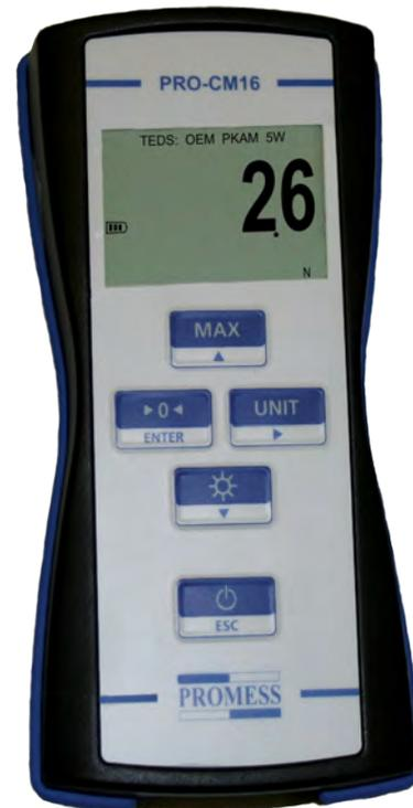
The PRO-CM16 is a battery operated handheld meter with a precision amplifier housed in a very robust enclosure. The meter is designed to work with Promess transducers and standard strain gauge load cells to calibrate and certify force and torque measuring systems.
